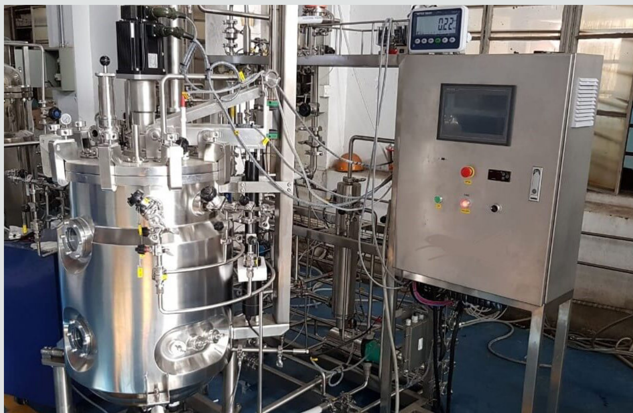
Bioreactor for cell culture 100 I, with OD detection (Egypt).
