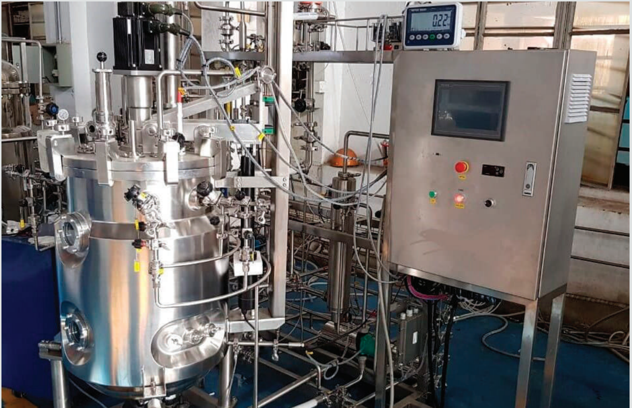
Bioreactor for cell culture 100 l, with OD detection (Egypt).
